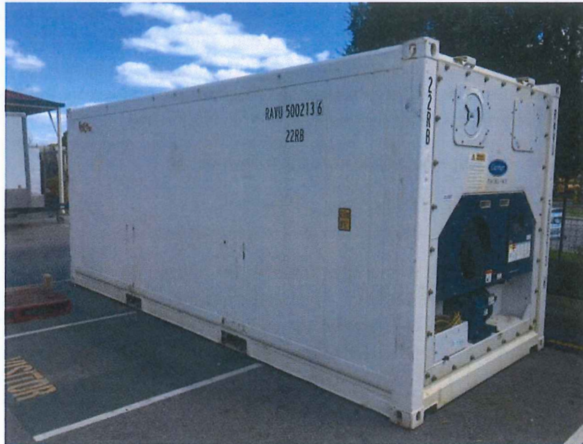
Figure 3: Image of proposed refrigerated container, with the motor featured towards the bottom right.
