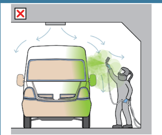
FIGURE 7 The operator is exposed to overspray and stretching and reaching can cause discomfort and injury.
