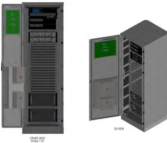
Figure 6: Example of a 4-Bay Outdoor Ground Equipment Cabinet
