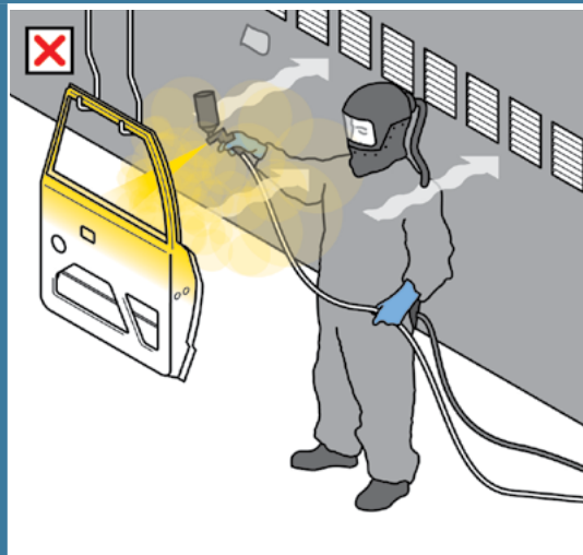
FIGURE 3 Spraying with a 'short' nozzle may cause overspray of the operator.
